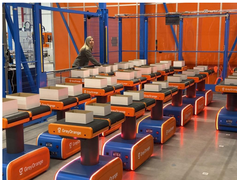
Bron: Active Ants E-fulfilment - Picking port AMR
